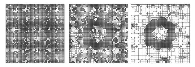
Obr. 3. On the left: the initial grid (12 658 elements). In the middle: the grid in the 4th scale step (9835). On the right: the final grid (the  $10^{th}$  time step with 4615 elements).
