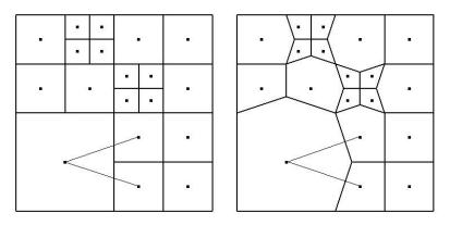
Obr. 1. An example of the original quadtree grid together with the representative points of its elements (on the left). This grid is transformed into the consistent one (on the right).
