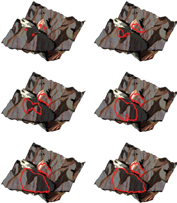
Fig. 16 Large-scale simulation in the area of Staré Hory in central Slovakia, considering heterogeneous fuel and northwest wind ( 315^\circ ) at speed 8 \text{ mmin}^{-1} . Initial condition is given by 4 circles in the horizontal projection
