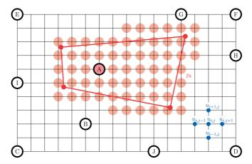
FIGURE 2.5. Illustration of the discretization of the computational domain  $\Omega$  and approximation of our mathematical model in cases A – J. By pink color we plot the grid nodes in the outer discrete envelope  $E(p_k)$  of the polygon  $p_k$  (plotted in red), where we consider Dirichlet conditions. In case B we consider the standard approximation of the Laplace equation while in cases C–J we consider its adjustment at the boundary  $\partial\Omega$ .
