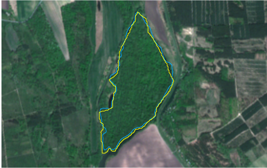
FIGURE 13. Semi-automatic segmentation (yellow) and GPS track (light-blue) with almost exact overlap. The maximal Hausdorff distance is 62.1m and the mean Hausdorff distance is 14.0m in this case, which means that we obtained almost the pixel resolution (10m) accuracy.
