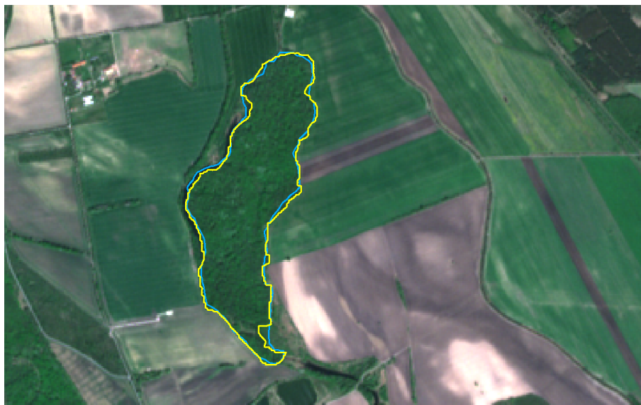
FIGURE 14. An example of a complicated border of the riparian forest. We compare the semi-automatic segmentation (yellow) and GPS track (light-blue). The mean Hausdorff distance is 12.0m and the maximal Hausdorff distance, in this case, is 62.1m, indicating correctly discrepancy in habitat area estimate in the field and by employing the Sentinel-2 optical data.
