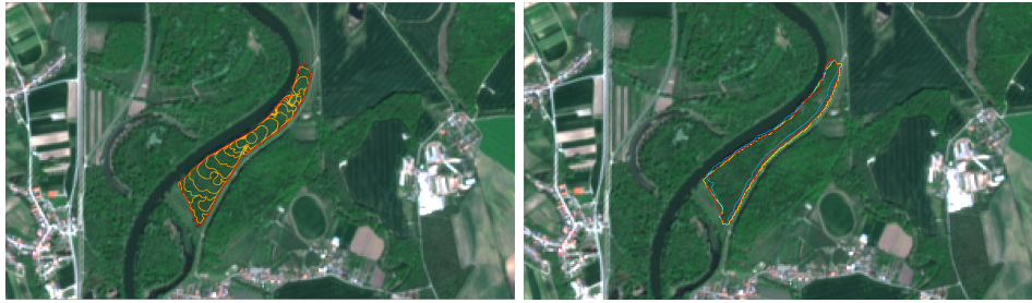
FIGURE 6. Left: the evolution of the segmentation curve from the initial circle to the final state. Right: the final automatic segmentation (red) together with the result of the semi-automatic segmentation (yellow) and the GPS track (light-blue).
